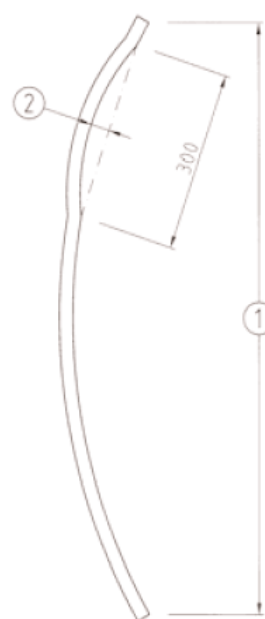
Figure A.1 — Representation of local distortion
