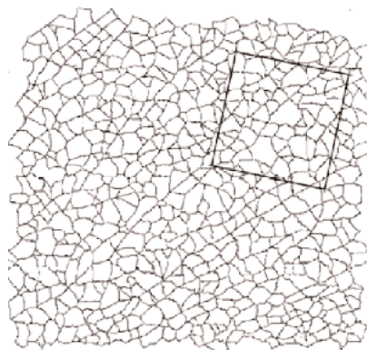
Figure C.1 — Select the area of coarsest fracture, according to 11.4, place the template on the test specimen and draw round the template.
